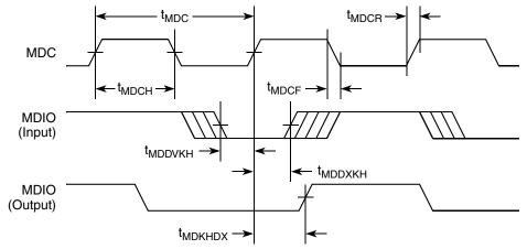
Figure 26. MII Management Interface Timing Diagram
