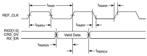
Figure 25. RMII Receive AC Timing Diagram
