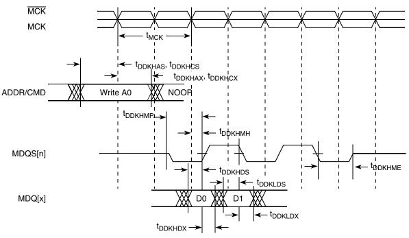
Figure 5. DDR and DDR2 SDRAM Output Timing Diagram
