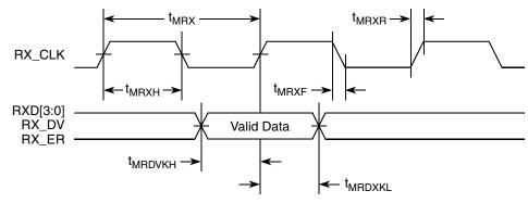
Figure 18. MII Receive AC Timing Diagram
