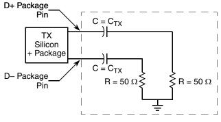
Figure 58. Compliance Test/Measurement Load
