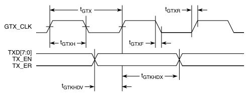
Figure 13. GMII Transmit AC Timing Diagram
