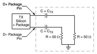
Figure 10. SGMII AC Test/Measurement Load
