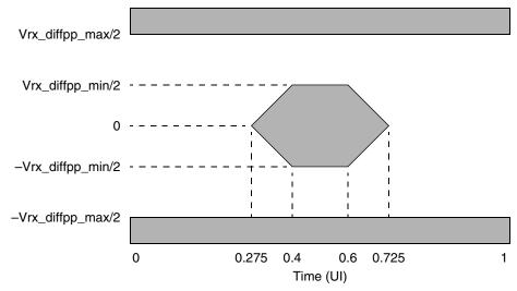
Figure 9. Receive Input Compliance Mask
