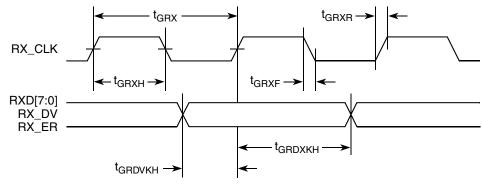
Figure 15. GMII Receive AC Timing Diagram
