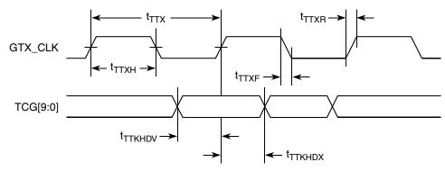
Figure 19. TBI Transmit AC Timing Diagram
