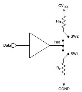
Figure 67. Driver Impedance Measurement
