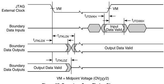
Figure 37. Boundary-Scan Timing Diagram
