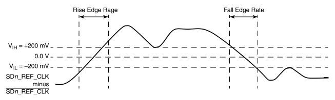
Figure 53. Differential Measurement Points for Rise and Fall Time
