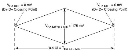
Figure 57. Minimum Receiver Eye Timing and Voltage Compliance Specification
