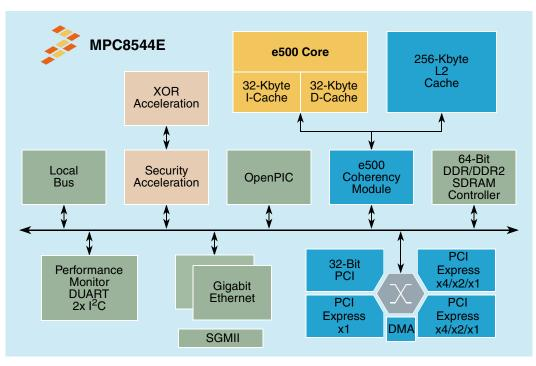
Figure 1. MPC8544E Block Diagram
