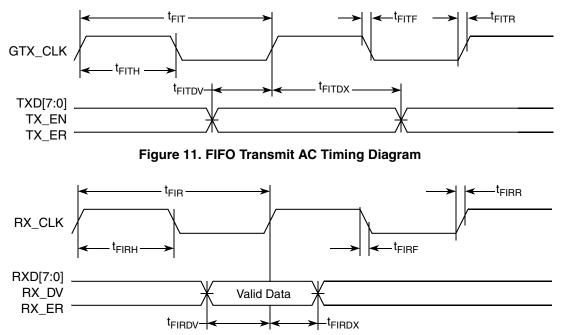
Figure 12. FIFO Receive AC Timing Diagram
