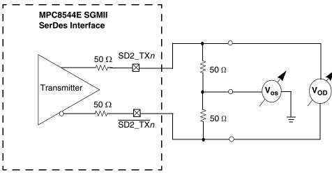
Figure 8. SGMII Transmitter DC Measurement Circuit
