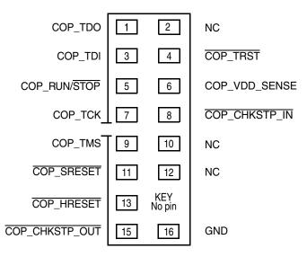
Figure 68. COP Connector Physical Pinout
