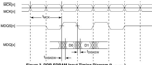
Figure 3. DDR SDRAM Input Timing Diagram (t<sub>DISKEW</sub>)
