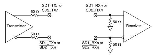
Figure 55. SerDes Transmitter and Receiver Reference Circuits
