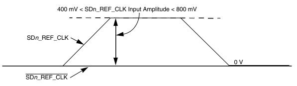
Figure 48. Single-Ended Reference Clock Input DC Requirements
