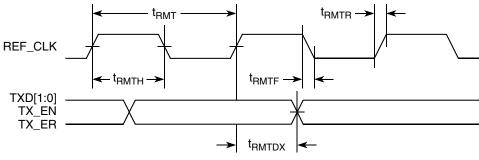
Figure 23. RMII Transmit AC Timing Diagram
