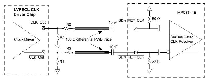
Figure 51. AC-Coupled Differential Connection with LVPECL Clock Driver (Reference Only)
