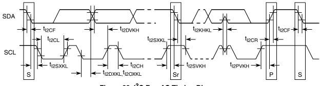
Figure 39. I<sup>2</sup>C Bus AC Timing Diagram
