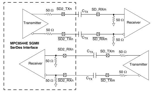
Figure 7 shows an example of a 4-wire AC-coupled SGMII serial link connection.
