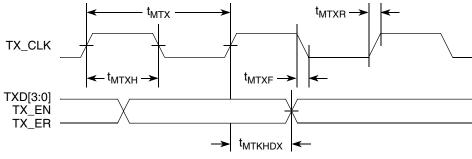
Figure 16. MII Transmit AC Timing Diagram
