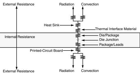
(Note the internal versus external package resistance.)
