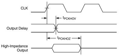
Figure 43. PCI Output AC Timing Measurement Condition
