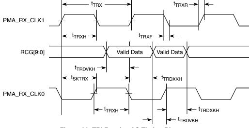
Figure 20. TBI Receive AC Timing Diagram
