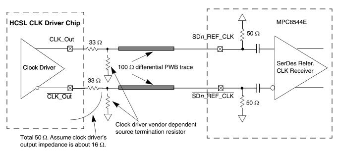
Figure 49. DC-Coupled Differential Connection with HCSL Clock Driver (Reference Only)
