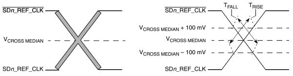
Figure 54. Single-Ended Measurement Points for Rise and Fall Time Matching
