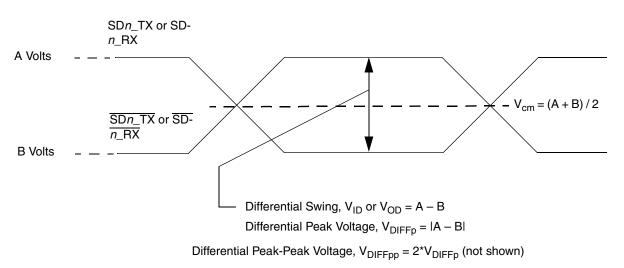
Figure 44. Differential Voltage Definitions for Transmitter or Receiver
