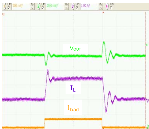
Figure 15. MODE=1, 100 mA to 1.5 A to 100 mA, 5 \mu\text{s}/\text{div} .
