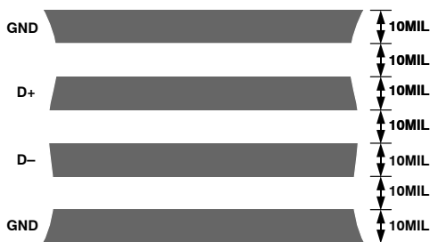
Figure 18. Arrangement of Signal Tracks
