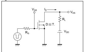
Fig. 2-1 GATE CHARGE MEASUREMENT CIRCUIT
