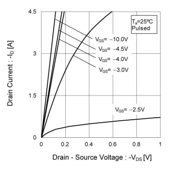
Fig.6 Typical Output Characteristics(II)
